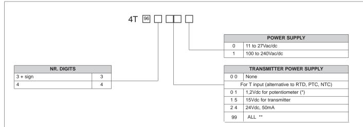
(\*) R77 for version with potentiometer input (Rinput >  $10M\Omega$ )
