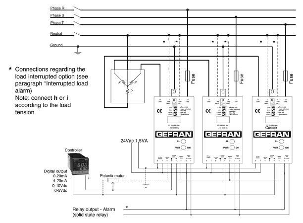
Three-phase connection (triangle or star) without neutral, with control of two phases using one GT in Master configuration and one GS in Slave configuration.
