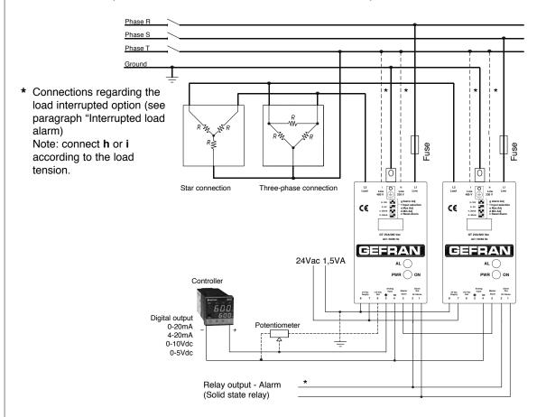
Star or delta three-phase connection without neutral, with control of three phases.
