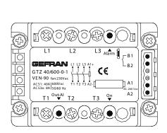
Phase 1 input 11. L2: Phase 2 input L3: Phase 3 input T1: Phase 1 output T2: Phase 2 output T3: Phase 3 output Control signal (AC) A1: Control signal (AC) A2: B1: Alarm output (option) R2· Alarm output (option) Led ON: Red led signal indicator
