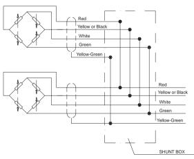
In systems that use several cells, the parallel connection automatically sums the loads on each individual cell.
