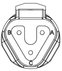
Every connector has a protection rating IP69K/IP67 with female connector properly installed
