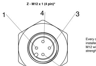
Every connector has a protection rating IP69K/IP67 with female connector properly installed.
