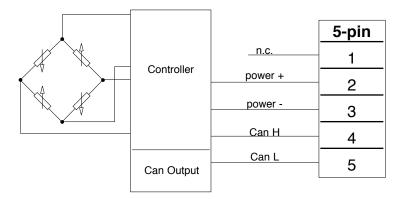
Shielding is connected to transducer body. It is advisable to ground it on the instrument side as well
